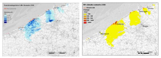
Figure 12: Results of the flood risk calculations for an extreme storm for the M+ 2100 scenario. Left: water depth, right: total damage.
