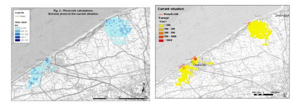
Figure 11: Results of the flood risk calculations for an extreme storm in the present situation. Left: water depth, right: total damage.
