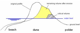
Figure 10: Evaluation of remaining volume compared to critical volume
