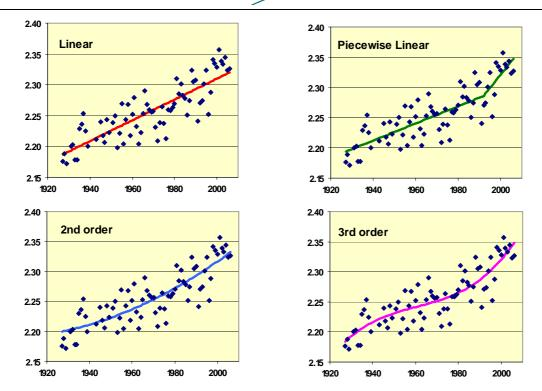
Figure 3: Trend analysis of relative mean sea level at Oostende over the period 1927-2006. (Top left: linear regression; top right: piecewise linear; bottom left & right: 2nd order and 3rd order polynomial models)
